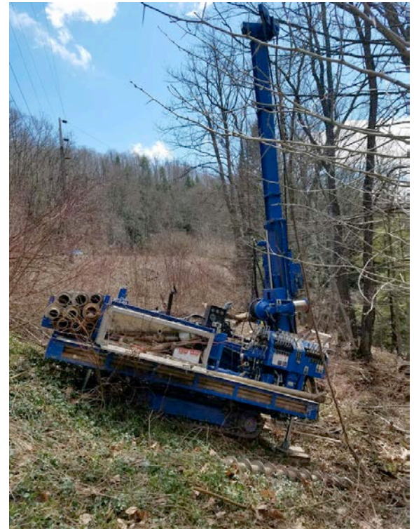
Geotechnical drill rig used for slope stability analysis.
